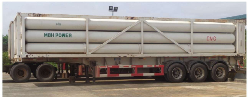
CNG TUBE SKID
